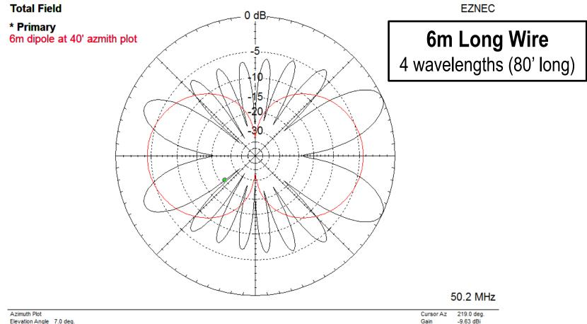
Elevation Angle 7.0 deg. Outer Ring 12.35 dBi 219.0 deg. -9.63 dBi -21.98 dBmax
