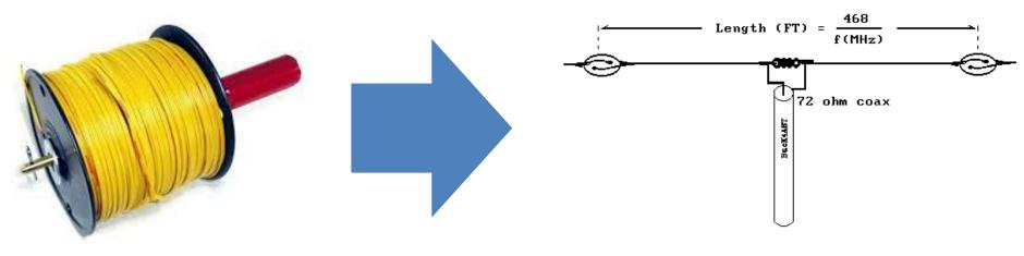
A dipole is a half-wave antenna fed at the center. The impedance at the center is near 72 ohms.
