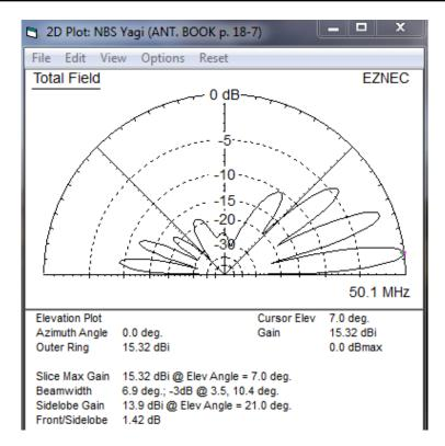
Source 1 Voltage = 12.8 V at 23.48 deg. Current = 1 A at 0.0 deg. Impedance = 11.74 + J 5.101 ohms Power = 11.74 watts SWR (50 ohm system) = 4.305 (75 ohm system) = 6.418
