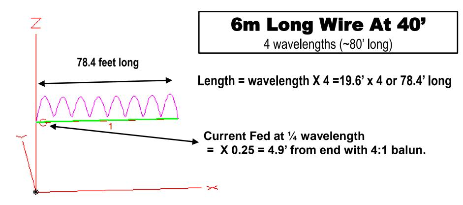
Voltage = 144.1 V at 1.87 deg. Current = 1 A at 0.0 deg. Impedance = 144 + J 4.691 ohms Power = 144 watts SWR (50 ohm system) = 2.884 (200 ohm system) = 1.390
