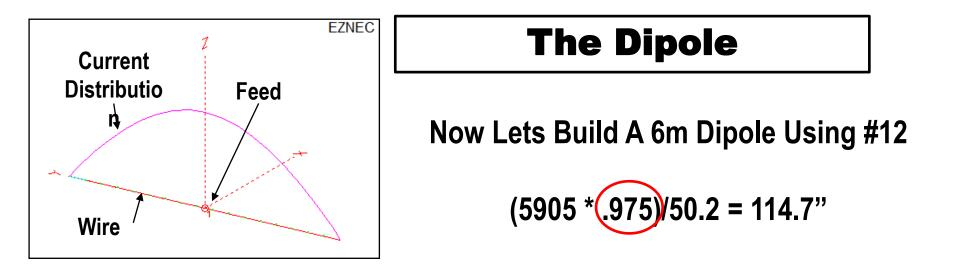
Voltage = 76.29 V at 10.94 deg. Current = 1 A at 0.0 deg. Impedance = 74.9 + J 14.48 ohms Power = 74.9 watts SWR (50 ohm system) = 1.594 (75 ohm system) = 1.213
