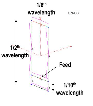
Voltage = 87.76 V at 1.7 deg. Current = 1 A at 0.0 deg. Impedance = 87.72 + J 2.601 ohms Power = 87.72 watts SWR (50 ohm system) = 1.757 (75 ohm system) = 1.173
